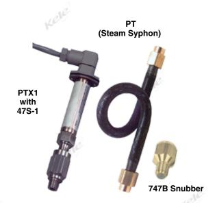
The **Model PT** is constructed of steel and is suitable for steam pressure to 250 psig (1724 kPa) 400°F (204°C). Each is furnished with two 1/4" FPT x 1/8" FPT couplings and one 1/8" MPT x 1/8" MPT nipple for convenient installation.
